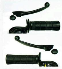
All of the braking with Beluga is done by hand. The right hand operates the front brake and the left one, the rear. Again, it frees the rider's mind from having to think about hand and foot co-ordination and allows total concentration on the road. This is a safety feature that will be particularly appreciated by new riders. Both drum brakes are waterproof and dustproof.
