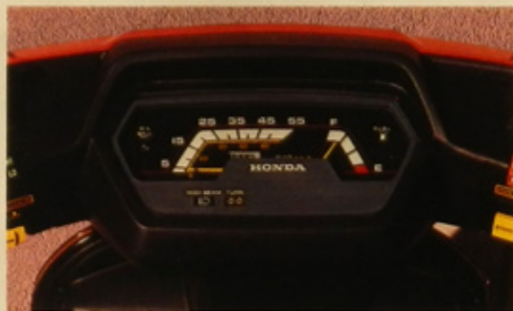
Complete instrumentation includes speedometer, odometer, fuel gauge and low-oil warning light.
