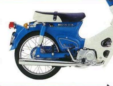
The bigger brother to the C50, the C70 is equipped with a more powerful 70cc, overhead camshaft, four- stroke engine.
