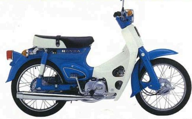
The automatic choice in step-thru's. This moped styled version based on Honda's world famous 4-stroke C50 features a fully automatic smooth as silk transmission, step-thru frame design, 12 volt electrics, powerful lighting system, large dual soft padded seat, pillion footrests, leg shield protection, twin rear view mirrors and full front and rear suspension. Dimensions: length 1800mm, width 660mm, height 1010mm. Fuel capacity: 4 litres.
