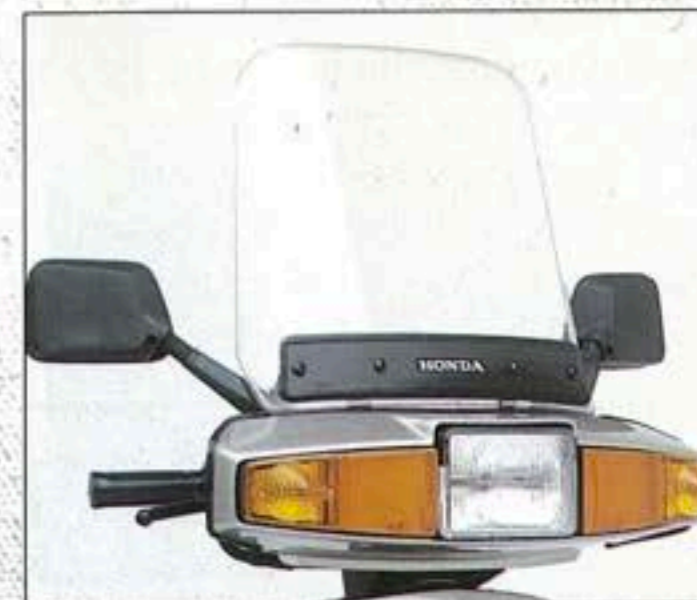
Headlight/signal light housing incorporates instrument panel. Optional windshield looks good and adds protection.
