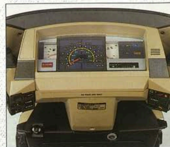
Easy-to-read, automotive-style instrument panel includes a fuel gauge and service reminder.
