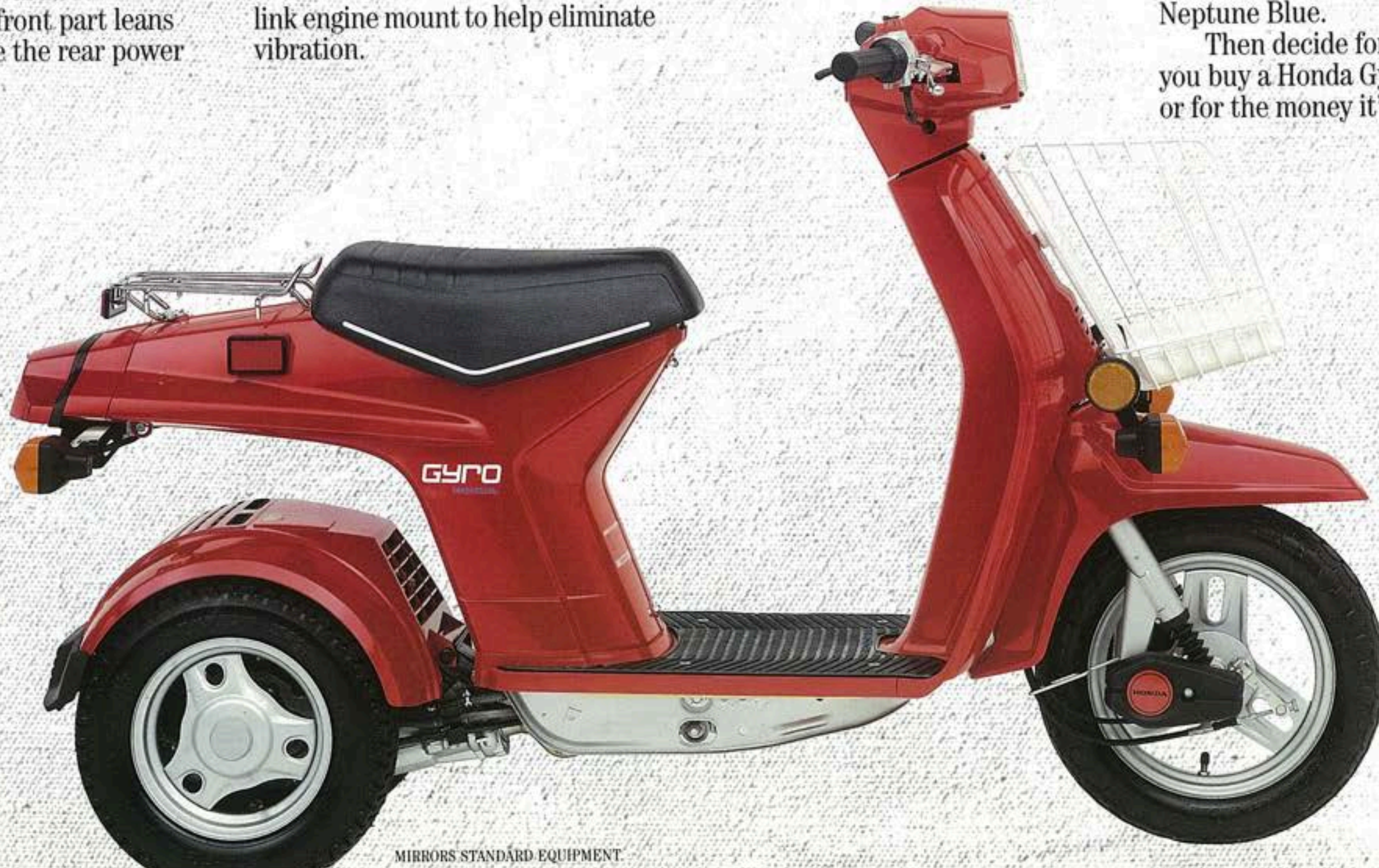
New "hinge-in-the-middle" design lets you lean front section into corners, while rear wheels remain flat on road.
