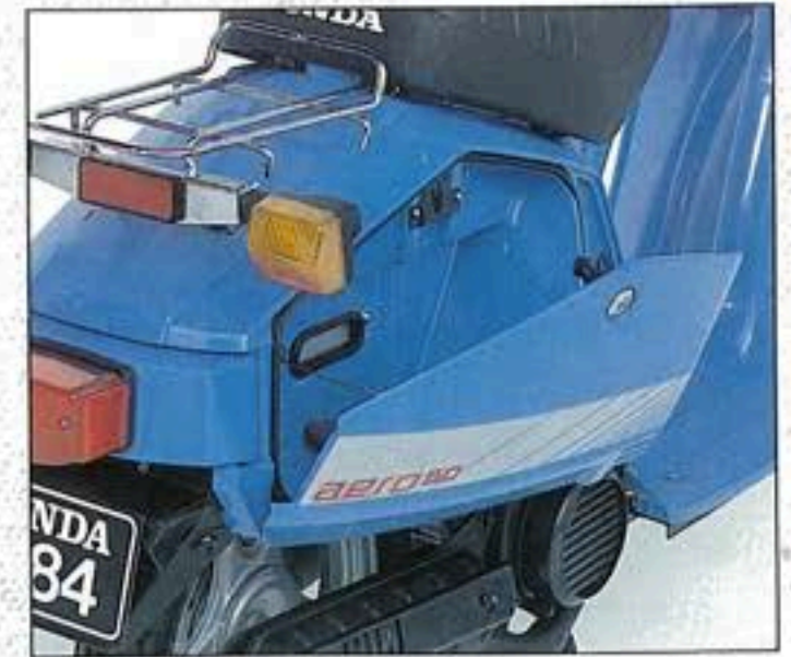
A locking side compartment under the seat holds valuables.
