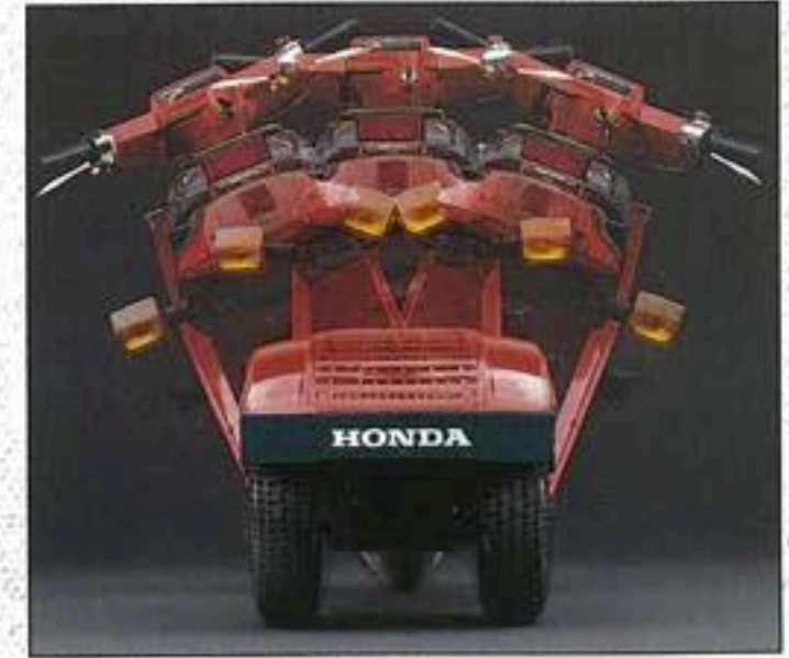
New "hinge-in-the-middle" design lets you lean front section into corners, while rear wheels remain flat on road.
