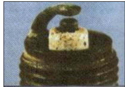
Fig. 91-Over heated spark plug
