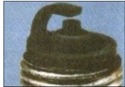
Fig. 89-Spark plug fouled with soot
