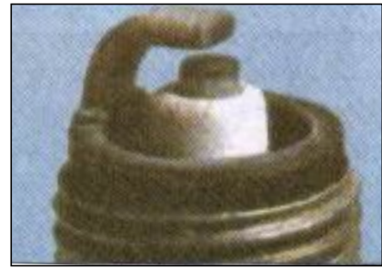
Fig. 88-Spark plug in normal condition
