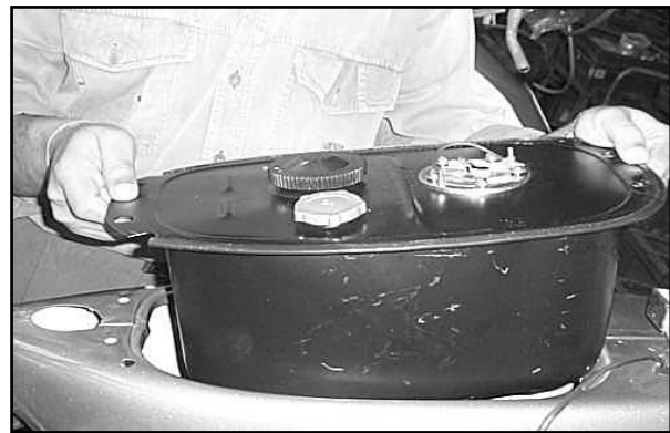
Fig. 185-Lifting out the tank from frame
