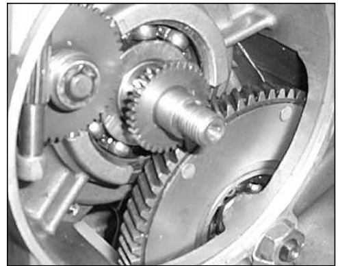
E.- Fit the drive gear and woodruff key
