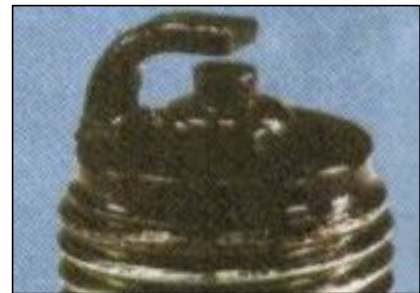
Fig. 90-Spark plug fouled with oil
